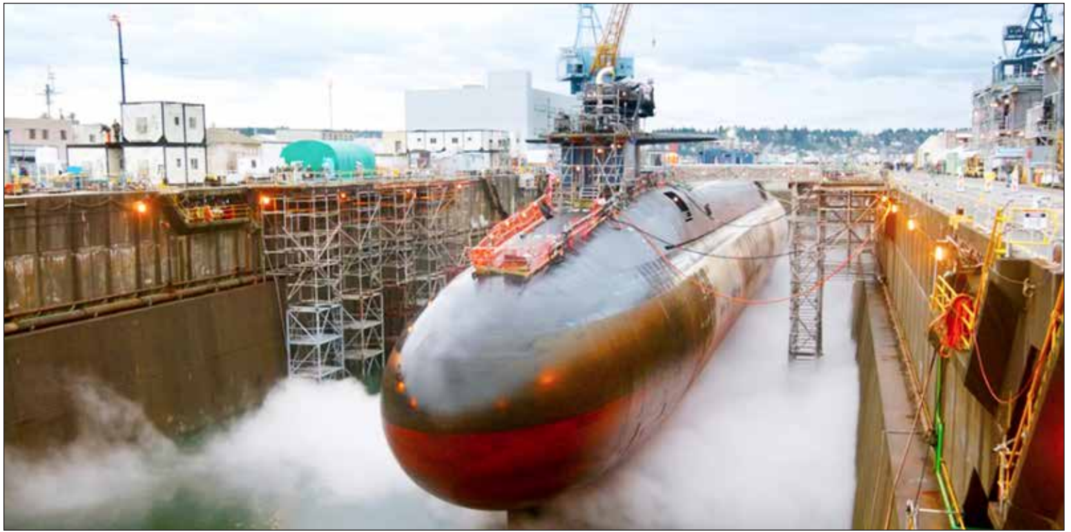
USS Ohio (SSBN-726) in a drydock during her conversion into a guided-missile submarine, August 14, 2003. (U.S. Navy photo.)
